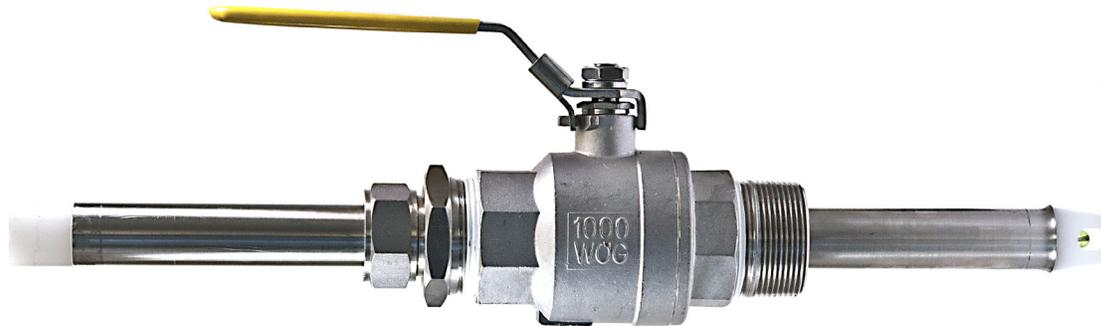
The LiveTap™ Insertion Assembly is ideal for use in areas where down time is critical by allowing removal of the electrode from a live line or tank without process interruption. Fitted with a 1.5" ball valve, the pH or ORP electrode can be removed for maintenance by sliding the 316L Stainless Steel sheath through the valve and closing it off. Your unit is now safe to remove.
